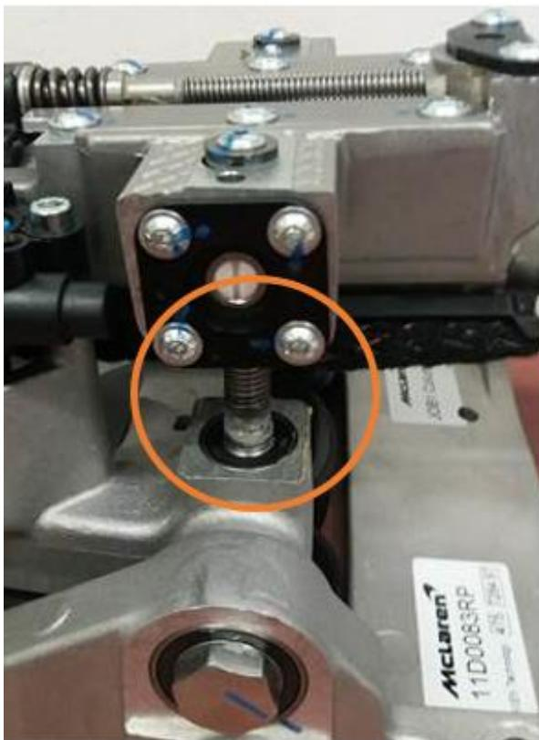
If the above has occurred, it can be identified by the steering column being in either full reach or rake position, not moving during the calibration and potentially be able to hear the motor attempting to drive the column but after 2 to 3 attempts it will stop.
